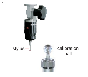
standard probe set ( optional ), includes Ø2mm and Ø3mm styli, Ø25mm calibration ball, measuring accuracy is 10µm
